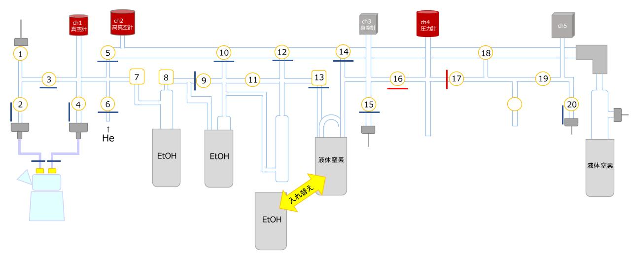
26. Replace the liquid nitrogen with ethanol. Do this quickly!
