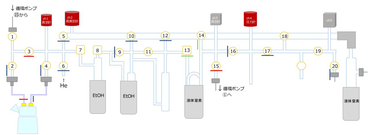
17. Turn off the circulation pump and close the center of the bubbling device (gas inlet).
