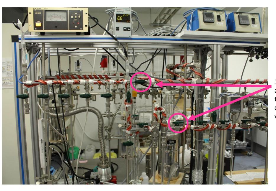
34. When the pressure stabilizes around 10^-3 to 10^-4, close the two valves on the graphite line to create a closed space for the high-vacuum pump.
